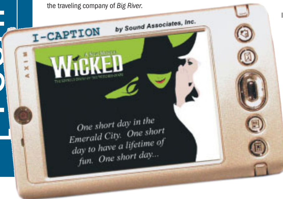
The I-Caption hand-held device (above), shown full size. Each image holds a few lines of dialogue. Wireless signals keyed to the show's lighting cues keep the dialogue synched up.
