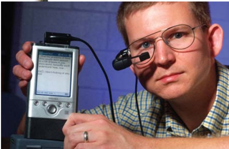
Left: Picture of the new Rear Window Captioning Reflector, developed and sold by Boston Light & Sound. It's said to be lighter and better able to hold its position. Below: The two primary components of the SightLine system: The PDA receives the captions wirelessly; and the tiny micro-display makes it seem like the captions are floating about 18 inches in front of your face.
